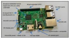
Figure 3. Raspberry Pi 3 Model B
